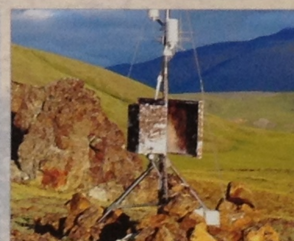
Figure 4. Evidence of high winds and flying debris/ice on station. Photo by Ken Hill - NPS.
